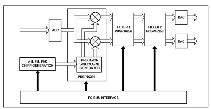
The evaluation system provides a complete environment for the development of high performance digital filtering and signal generation systems. The development system is based on the powerful Mitel Semiconductor's PDSP16350 and PDSP16256 digital signal processing components and comprises the following elements:
